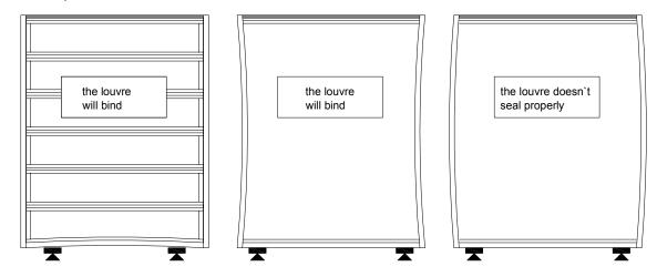
Incorrect installation can be identified by non-uniform joints between the blades and the side frame profiles. If screw-fixing through the vertical frame profiles, use the holes provided by the manufacturer (EuroLam) only. Anchoring fins can be screwed onto the outsides of the frame profiles for keyed connections. The anchors are fixed by additional screw-fixing with the frame.
